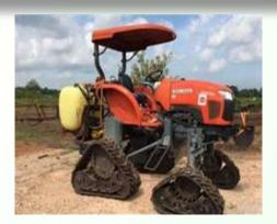
4 half track tractor- rubber typed
