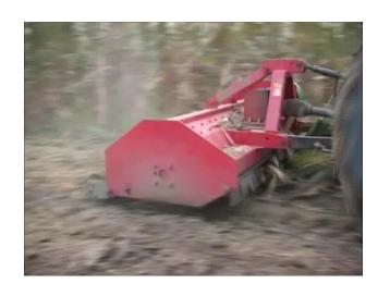
Powered shallow tillage to mix most stubble into surface soil 旋耕将较多秸秆混埋到地表以下
