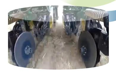
No stubble block; Narrow furrow; lower soil disturbance 圆盘开沟器,没有秸秆堵塞,开窄沟,动土量小
