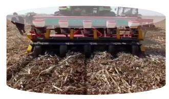
Use powered knife to do strip till and make a clean zone for the coming sowing 以驱动部件带状耕作土壤,没有秸秆堵塞,形成清洁播种带,进行播种
