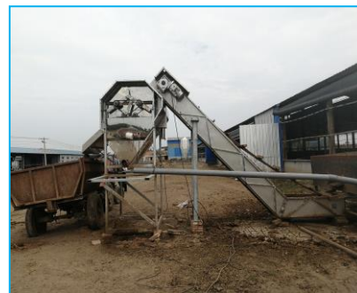
d) Dry-wet cow manure separation
