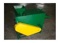
impurities and at the same time shriveled/immature, damaged and nonviable seeds are separated. Different grades of seeds are obtained by changing the sieves. High germination rates are achieved using cleaned and graded seed by this grader. The output capacity of this 0.746 kW electric motor driven machine is estimated as 150 kg/h in case of wheat.
