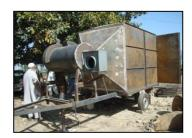
namely heating source (diesel burner), heating unit (heat exchanger), drying chamber, turmeric collectors (trays) and fan/blower. The drying capacity of the machine is about 1.5 tons per batch.
