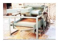
an output capacity of 0.5 ton/h with >98% cleaning efficiency.
