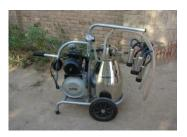
machine was tested on cows and buffaloes. It is capable to produce vacuum pressure upto 70 kPa. The vacuum pressure was adjusted to 44-46 kPa for water buffaloes and 42-44 kPa for cows. The pressure worked well for producing the required pulsation and continuous vacuum suction.
