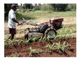
Use of two wheel tractor rotory as an inter-cultivator
