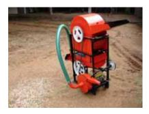
Two type of decorticators can shell the groundnut for consumption and also for seeds. Manual operated machine has the capacity of about 50 kg per hour and the electrical motor driven machine has fairly a large capacity.
