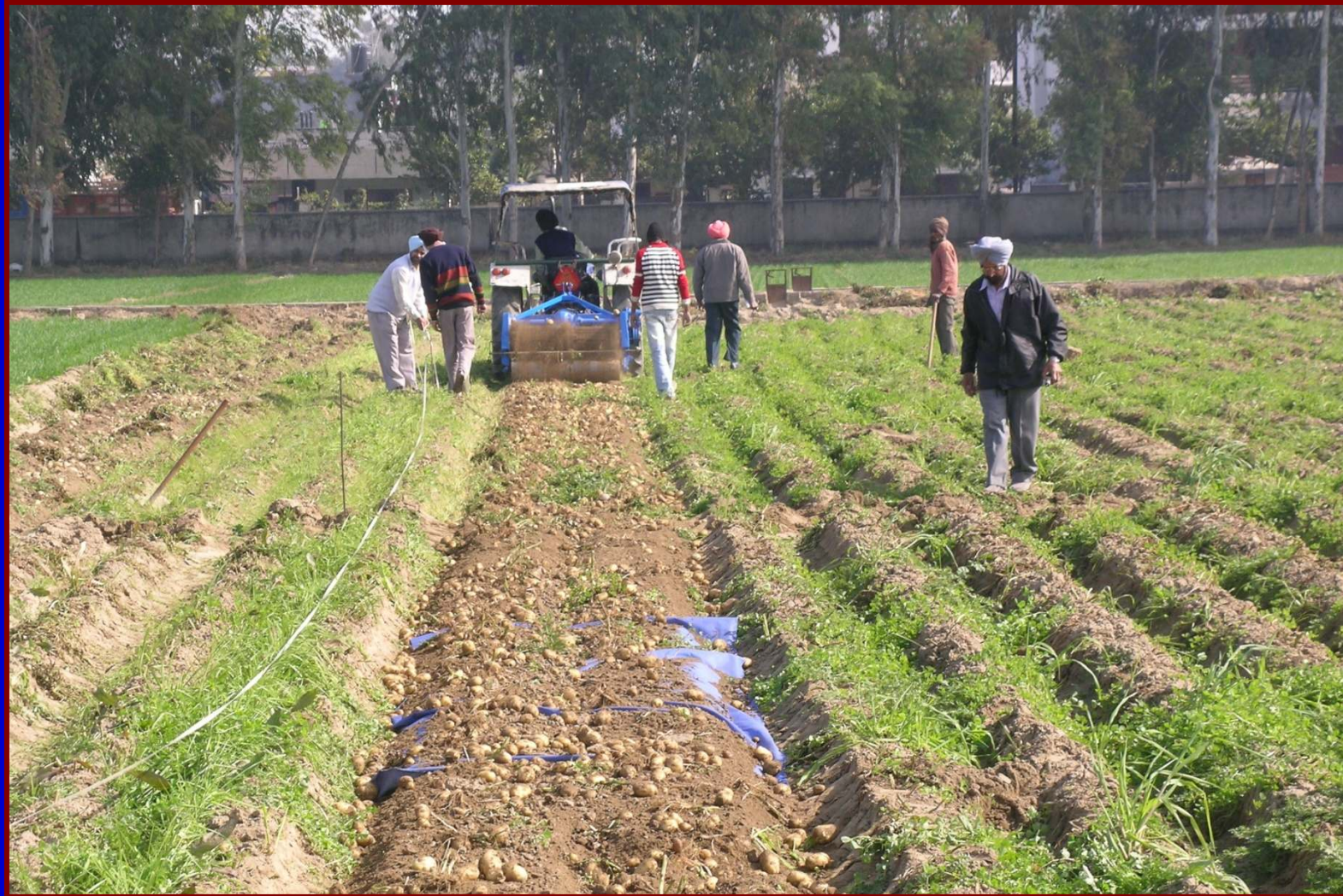
A view of root crop harvester in operation for digging potato
