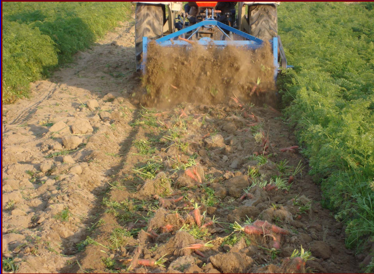
A view of root crop harvester in operation for digging carrot crop
