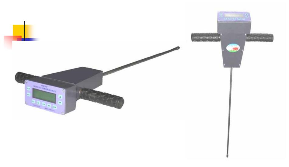
The handheld dual sensors have tested in different soil conditions and can be used simultaneously measure Soil moisture content, Cone index, penetration depth and position parameter with autodata storage
