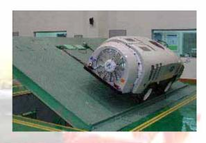
▲ Executing the turn-over test of off-road vehicles. The inspection of turn-over angle is performed by the local test method.
