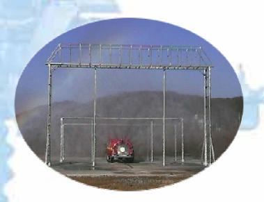
▲ Measurement of droplet coverage of speed sprayer
