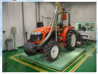
▲ Overall PTO performance of agricultural tractor such as power, torque, speed, fuel consumption, and specific fuel consumption is tested
