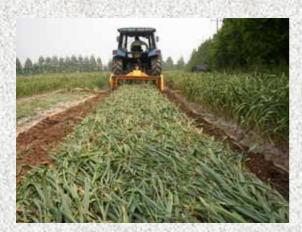
A electric-powered Leek harvester that cuts one row of leek and collects the leek plants in the harvesting box
