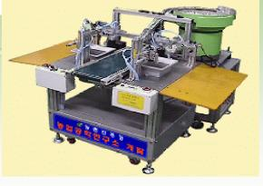
Grafting machine which can automatically carry out the series process such as cutting, joining, clipping, discharging for grafting gourd family vegetables
