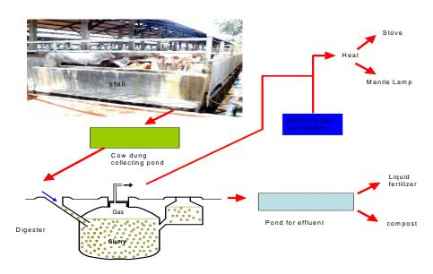
Figure 1. Schematic flow of Biogas Processing
