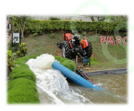
Very high capacity (more than 20,000 l/min.) four wheel tractor powered axial flow type water pump has been developed. It has very good demand in the Eastern Province. A number of manufacturers in that province were already trained. It consumed very low fuel per liter of water.
