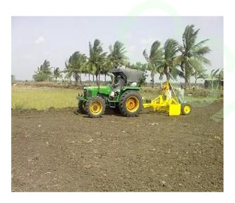
If land leveling is done with the use of laser guided land leveler both in lowland and highland about 20% - 30% water can be saved and also crop growing will be in uniform. The laser guider has to be imported and preliminary trials will be conducted.
