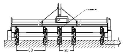
Fig. 5 Strip-tillage equipment.
