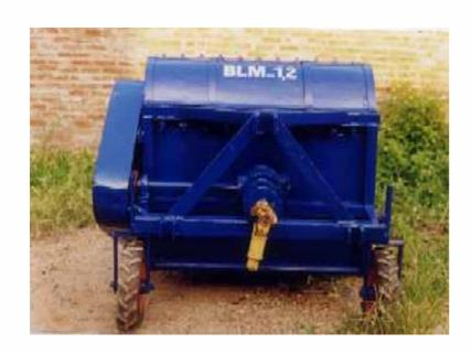
Fig. 4. Sugar-cane-leaf rotary chopper BLM-1.2
