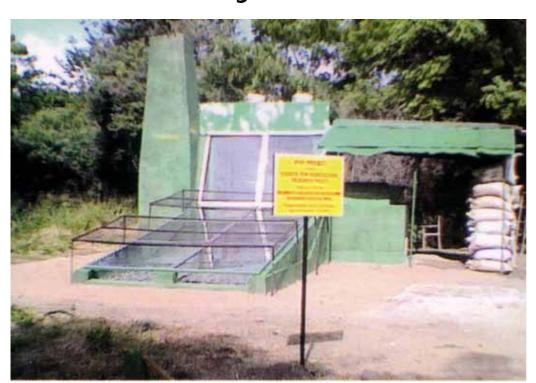
Solar Assisted Biomass fired dryer for dehydration of Agricultural Products
