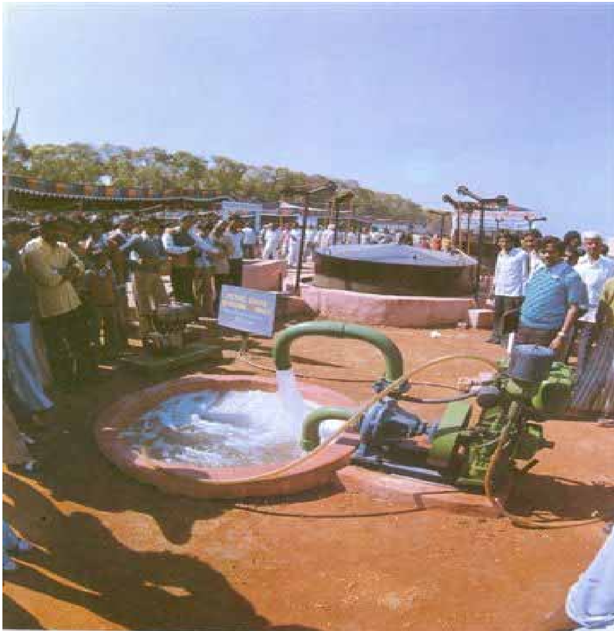
Biogas run Water Pump
