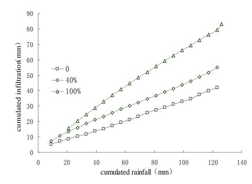
Fig1: Comparisons of Cumulated Seeping Quantity among Different Mulching Ratios
