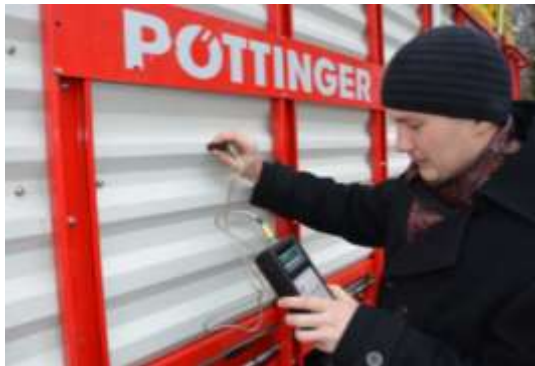
Assessment of the coating quality
