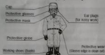
Spray worker wearing proper clothing
