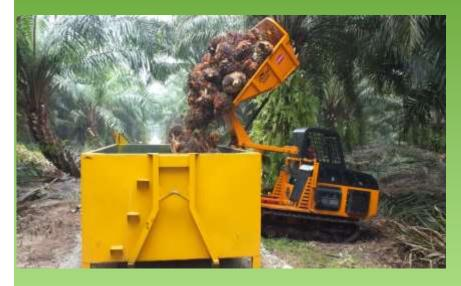
Jaguar X800, a 37HP multipurpose tractor was designed with a single chassis, compact and robust with the most efficient weight distribution ratio and the least ground pressure.
