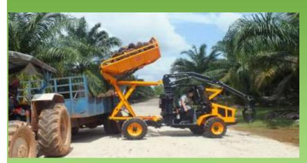
Tiger G1500 is capable of carrying 1500 kg of FFB payload, utilizing a minimal diesel fuel consumption of only 12 litres a day.
