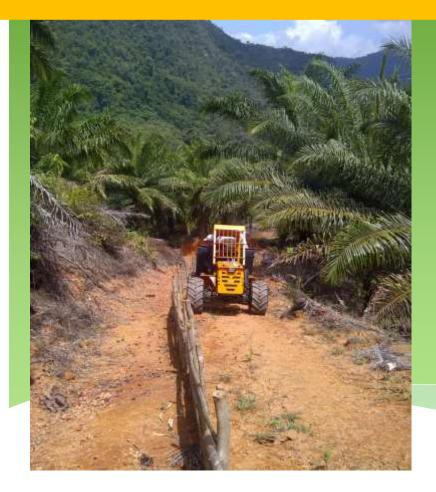
Rhyno is capable of carrying 700 kg of FFB payload, utilizing a minimal diesel fuel consumption of only 6-8 litres a day.
