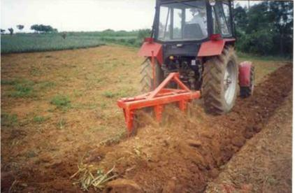
Soil Cultivation Machine for Sugar Cane Disk Harrow and Shank
