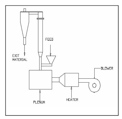
Schematic diagram of the AMDP Pneumatic Dryer
