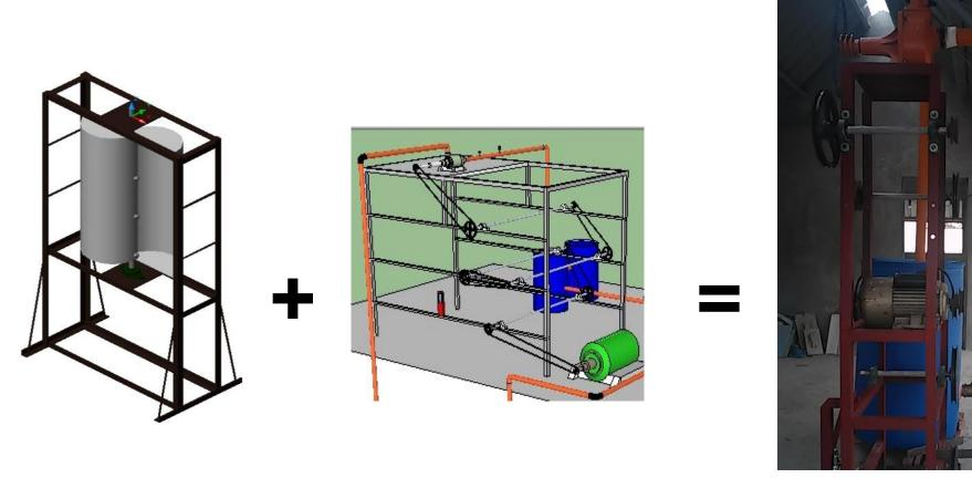
Wind pump system for supplemental irrigation
