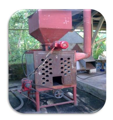
Thermal Energy for drying – Rice husks furnace for fruits and grain drying
