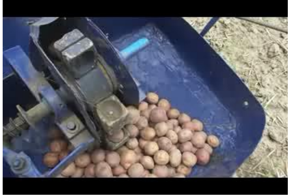
Power tiller driven potato planter
