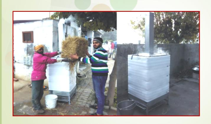
100 litres of water heated to 45-50°C in 3-4 hours
