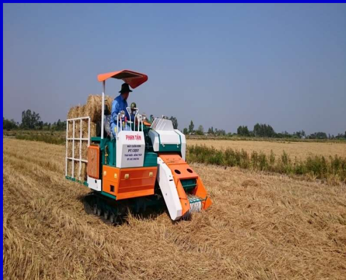
+ Local manufactured straw balers with a storing tank in the back: Phan Tan or Tu Sang mechanical enterprises
