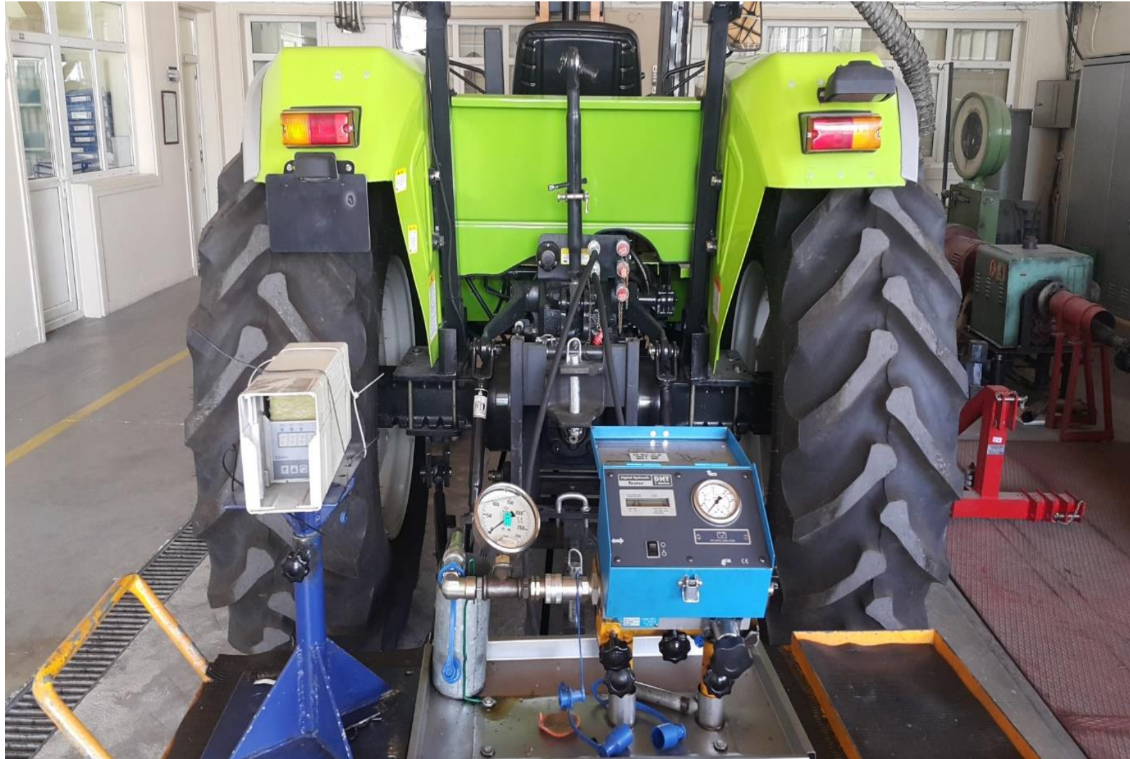
Hydraulic power and flow test
