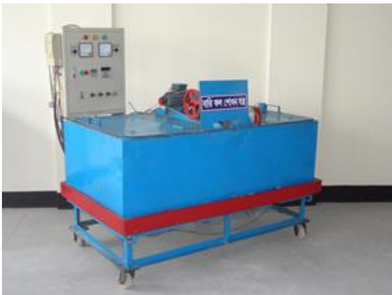
Hot water treatment plant
