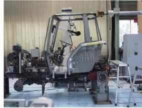
Static Load Test (at the rear end)
