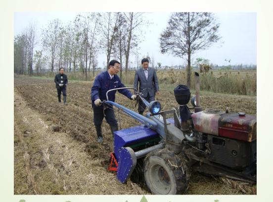
This machine has the functions of ploughing and sowing together, the tillage group and the planter are distributed on the same parallel lines.
