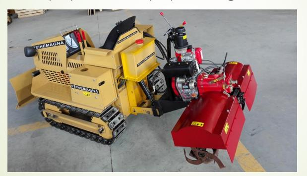
This machine is designed to cope with the comlex conditions of farmland in the mountainous area. Use of cartridge design, can be replaced within a few minutes to achieve a multi-purpose machines, reduce cost of purchasing machines for small holder farmers.
