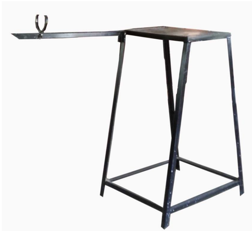
Figure 4a. Supporting Test Bench for Mounting Mister-Cum-Duster
