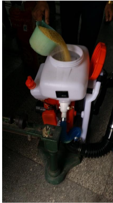
Figure 16a. Micro granules being filled while the duster is placed on a weighing scale
