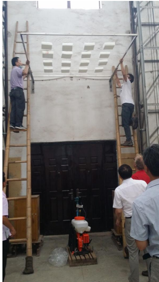
Figure 18a. Set up for vertical deposition test
